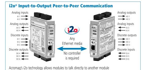
across any Ethernet media without a PLC, PC, or other controller in between. Input channels on one module can write to output channels on a remote module.
