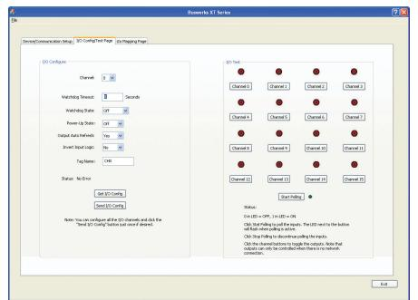
BusWorks XT software (download free from www.acromag.com) allows you to configure I/O modules offline with USB, save the file, and download settings into units later, at your convenience.
