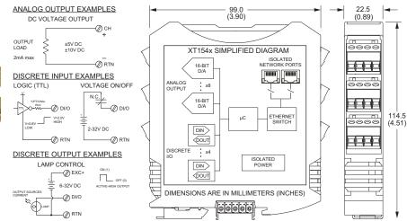
8 analog voltage outputs, 4 discrete I/O channels ◆ Modbus TCP/IP, Ethernet/IP, Profinet, or i2o communication
